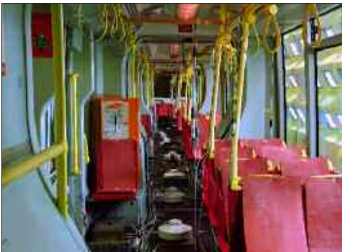
Figure 2: Installed equipment for passenger load simulation inside the ULF tram.
