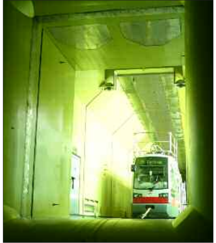
Figure 1: A ULF tram inside the climatic wind tunnel.
