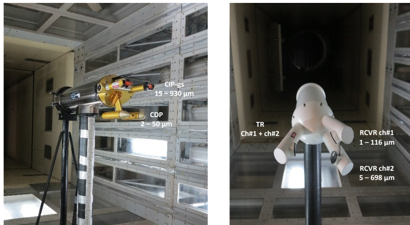
Figure 50: DLR CCP (Cloud Combination Probe) on the left, installed in the centerline of the CIRA IWT test section during the PSD/MVD measurement slot. CIRA 4D-PDI on the right installed with sample volume located on the centerline, in the same position of DLR CCP.
